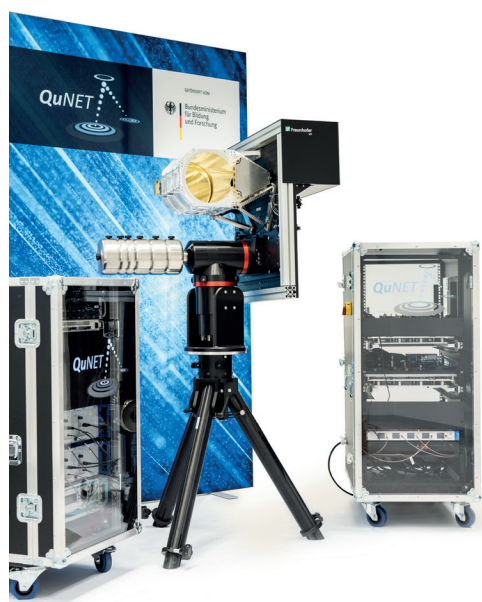
Optical transmitter with an high performance mirror telescope and an entangled photon source for intra-city links (experimental setup).
