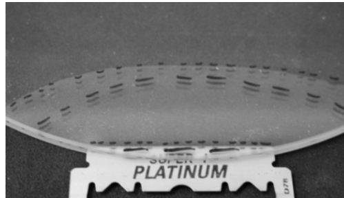
Figure 5: Applying the razor blade (Maszara) test to a bonded pair of ULE wafers
